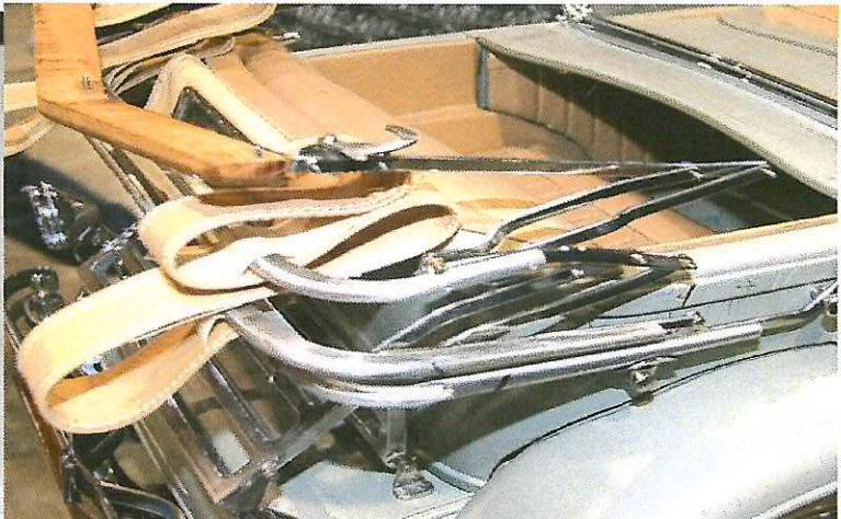
*The complicated convertible top mechanism is shown in the lowered position before the canvas top material was installed. Louis Chenot (Left) and Joe Martin (Right) inspect progress on the chassis and engine at the NAMES show in Detroit in 2007.*
